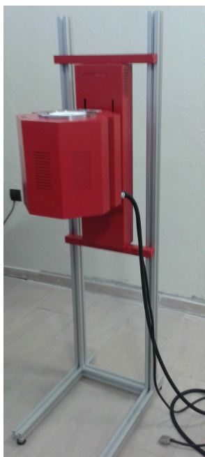
Model shown RCT-BW1_D5.2L23-1200 with optional mounting stand and electronically actuated Lifter.
